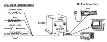
1) Voltage Spike Protection: Engine cranking, pump and motor operation send voltage "spikes" through a mobile electrical system that often "bulldoze" their way through the electronic circuitry. NAV-PAC eliminates this ruinous condition.
