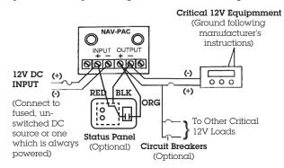
3) Optional Remote Panel: Mount in a conspicuous location where the loss of power indication will be noticed. The NAV-PAC will function normally without the remote panel or with the remote panel switch off. Connect the wiring as follows, see diagram. P/N 773-5037-0
