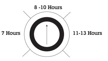
Note: Once the time-out circuit has put the charger into float mode, the charger will remain in this mode. Since the Phase Three Charger is well regulated, it is able to deliver its full rated output current in this mode and battery discharge will not occur (provided load current does not exceed charger rating and output wiring is properly sized).
