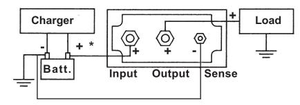
\* It is recommended to provide over-current fuse or circuit breaker protection on the ungrounded connection as close to the battery as possible.
