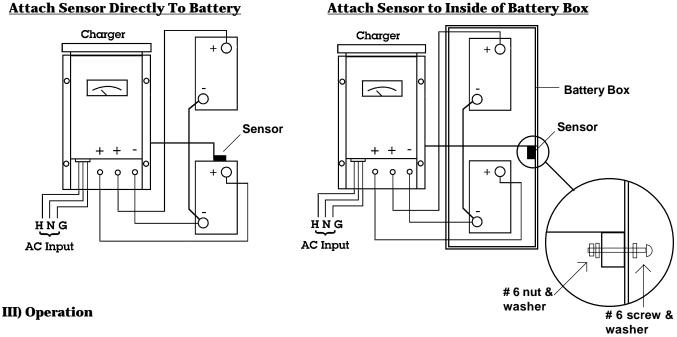
Once installed and plugged into the charger, the operation of the temperature sensor is automatic and no adjustments or maintenance are necessary. *Note: If the sensor should become unplugged for any reason, output voltages will be as shown at 72° in the chart below, regardless of actual battery temperature.*
