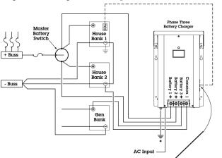
Optional Temperature Compensation Sensor. See page 8 for installation. Use provided cable clamps to secure probe caple
