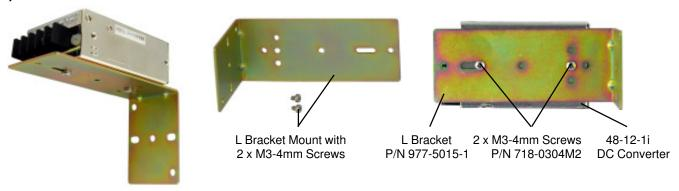
1) Mount the bracket to the converter using the M3-4mm x 2 screws; **DO NOT USE** the longer 6mm screws as this will damage the converter. 2) Now you can mount the converter and bracket to desired location. Hardware not supplied.
