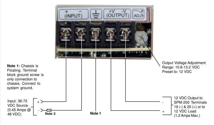
Note 2: Fuse hot side of input for wiring protection (fuse shown on negative input on a -48VDC input source).
