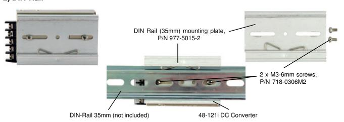
Use the M3-6mm screws to secure the DIN-Rail mounting plate to the side of the 48-12-1i converter. The mounting plate is slotted for adjusting its position, slide the DIN-Rail plate onto the DIN-Rail plate.
