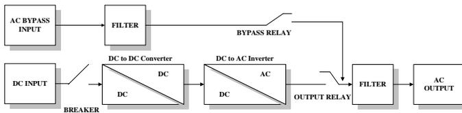
Rackmount Pure Sine Wave inverters feature IGBT (Insulated Gate Bipolar Transistor) technology, minimizing weight and dimension, while enhancing output short circuit reliability and overload capacity.
