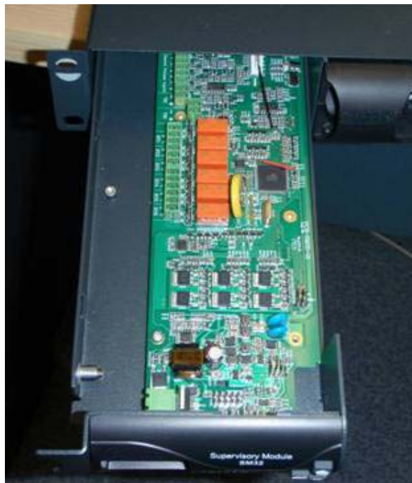
Fig 7. SM3x cable access
